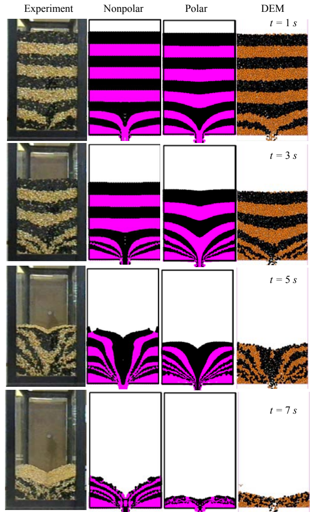
Figure 9. Corn flow patterns with the silo opening w = 45 \text{ mm}
